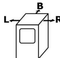
$$R = 200 \text{ mm} - L = 200 \text{ mm} - B = 50 \text{ mm}$$
